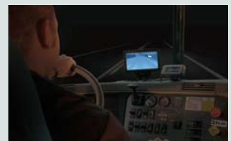
A monitor displaying the images of the PathFindIR, can be easily displayed on the dashboard. It quickly becomes a natural checkpoint for the driver similar to side view or rearview mirrors.
