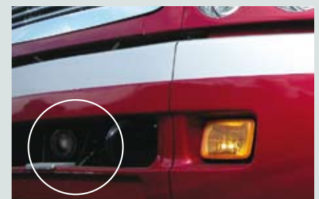
The PathFindIR installed behind the grill of a truck.
