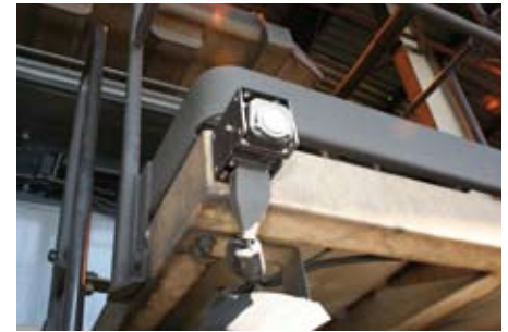
The PathFindIR thermal imaging camera can easily be mounted on front of a mining truck.
