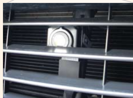
The FLIR Systems PathFindIR installed behind the vehicle grid of a Porsche Cayenne
