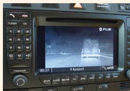
The thermal images generated by the PathFindIR can be displayed on any multi-function LCD display that accepts composite video. In this case on an LCD integrated in the Porsche dashboard.
