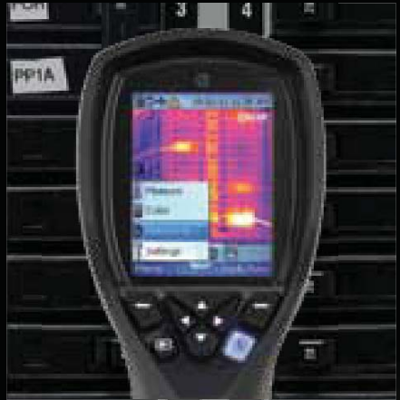
FLIR i3, temperature in 3,600 spots.
