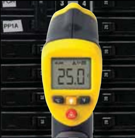
Spot pyrometer, temperature measurement in one spot.
