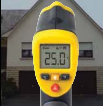
Spot pyrometer, temperature measurement in one spot.
