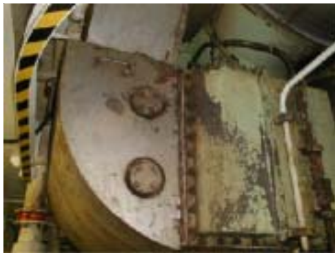
Main Engine Charge Air Cooler showing hot spots on seals
