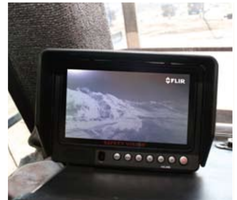
The thermal images produced by the PathFindIR are displayed on a large LCD display inside the trucks cabin. They help the driver to avoid accidents.
