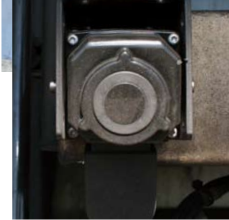
The PathFindIR thermal imaging camera can easily be mounted on front of a mining truck.
