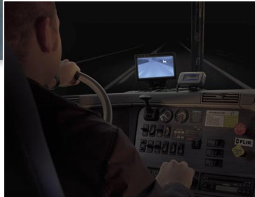
A monitor displaying the images of the PathFindIR, can be easily displayed on the dashboard. It quickly becomes a natural checkpoint for the driver similar to side view or rearview mirrors.
