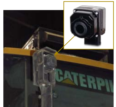
The FLIR Systems PathfindIR installed on the wheel loader.
