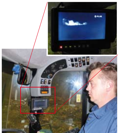
The thermal images of the FLIR Systems PathFindIR are displayed on the same LCD as the images of the reversing camera. Note the hot spot in the thermal image which clearly shows a part of the waste pile that was turned.
