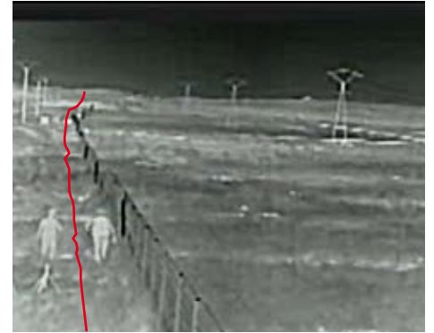
FLIR Sensors Manager contains video analytics algorithms like Trip Wire. An alarm will go off if someone crosses the line set by the operator.
